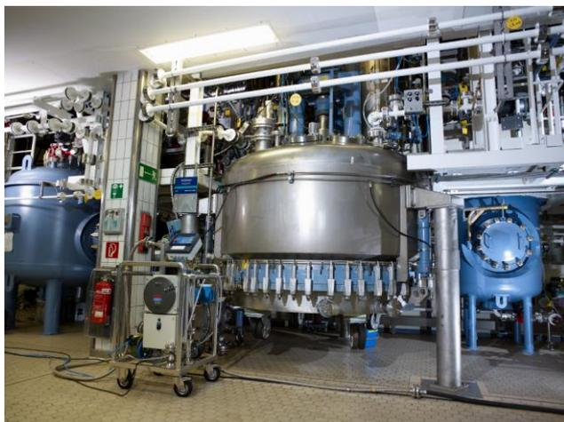
Cleaning of a nutsche filter in the Plant 3 of Saltigo GmbH in Leverkusen. Thanks to the 2.5 square meter filter area, approximately 800 kilograms of product can be filtered per operation. Photo: Saltigo GmbH
