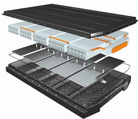
The demonstrator was developed based on the battery housing of a C-segment electric vehicle. It consists of a housing tray with crash structure, a housing cover and an underrun (underbody) protection.
